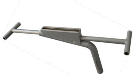
Figure 3: Sampler for hydro-mixture
