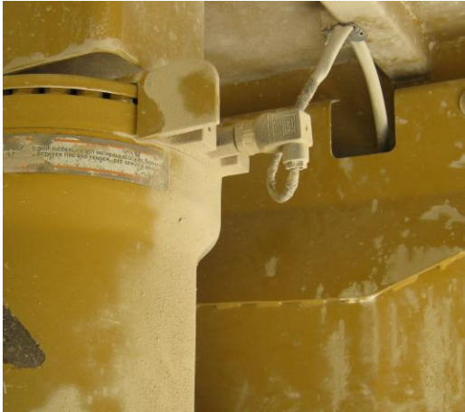
Figure 1. Front shock absorber of CAT 771D sensor mounted
