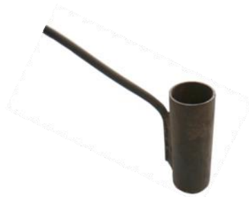
Figure 1: Sampler for dry ash
