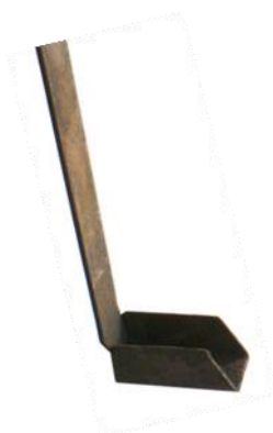
Figure 2: Sampler for slag
